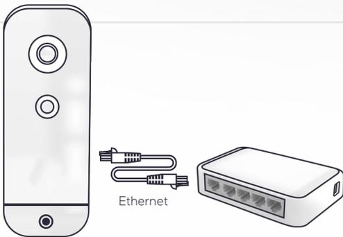
Connect to your door hardware (e.g., electronic locks, door contacts, etc.) and plug reader into a PoE switch to power it up.
