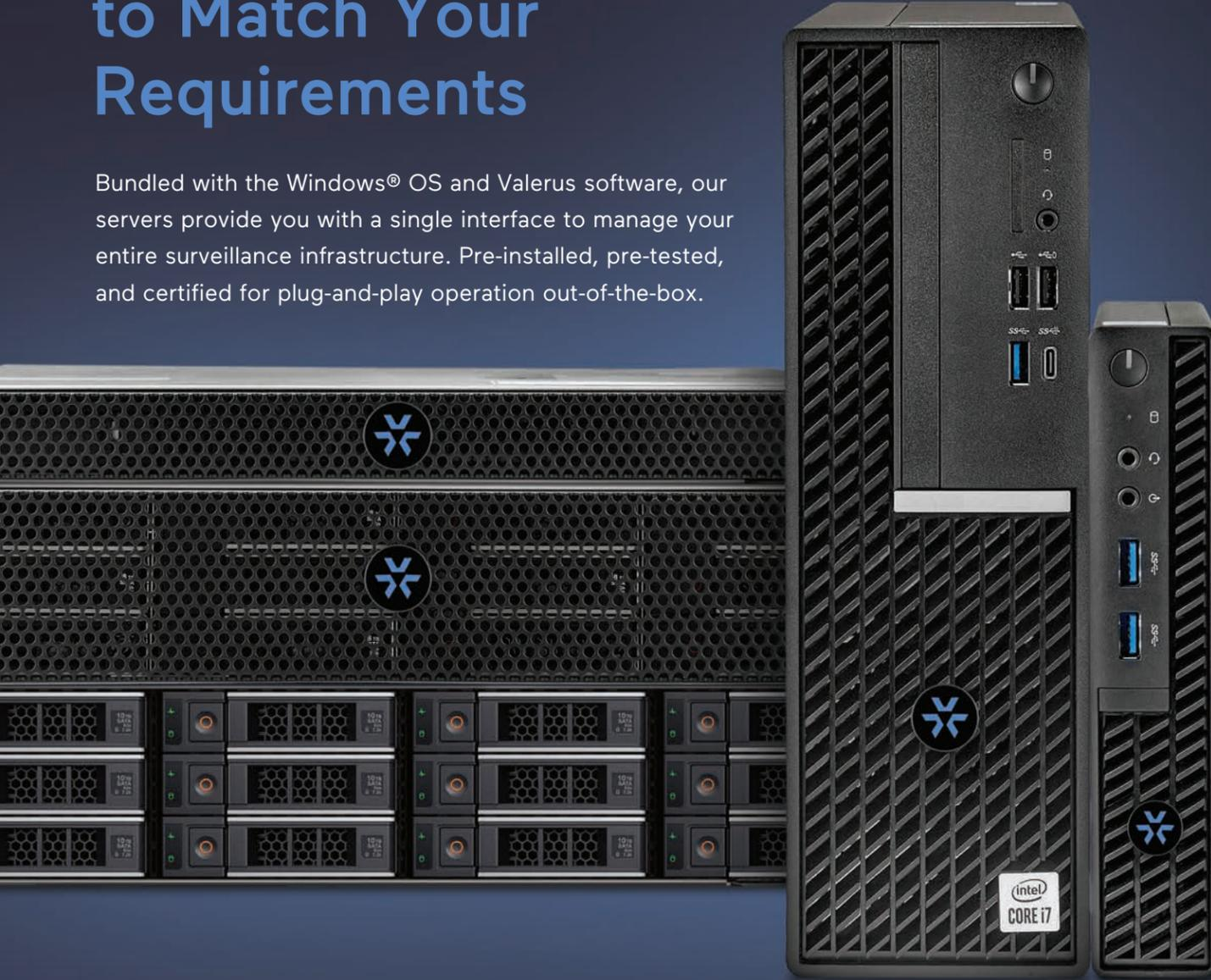
**Recording Servers** communicate, stream, and record video and audio from the edge devices.
