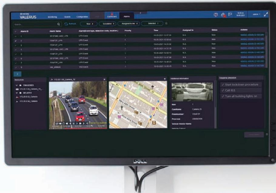
You can configure alarm inputs (like intrusion) to automatically trigger relay outputs (like a door strike) in response to critical situations (like a perimeter breach).
