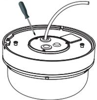
**Step 8:** Assemble camera with cap first. The ▽ should be aligned with OPEN (□).
