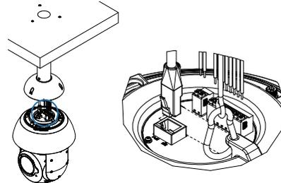
5. Attach the camera and pendant mount [align (D) with (E)].
