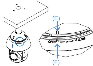
6. Rotate the camera in the CLOSE direction and then tighten screws (provided) (3x) to fix the camera on the Cap.
