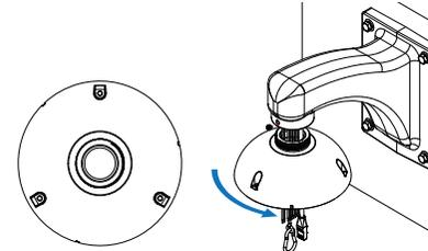
3. Hook the other end of the safety wire on (D). Connect the cable with terminal block and plug-in the corresponding holes and RJ-45 connector.
