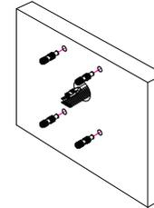
The safety wire has 2 hooks, one at each end. Hook one end of the safety wire (A) on the wall mount and pull the cable through the wall mount; fasten screws to secure the wall mount on the wall.
