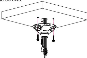
3. Fasten the tube and Cap, aligning B (one of the holes in Cap) with A (the hole in tube). Tighten the hexagonal screw (A) with proper tool.
