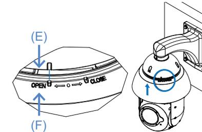
5. Rotate the camera in the CLOSE direction and then tighten screws (provided) (3x) to fix the camera on the Cap.
