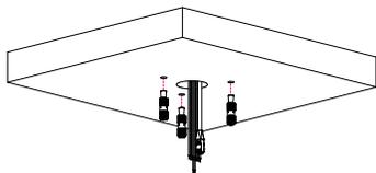
2. Pull the safety wire and cables through the bottom case of pendant mount and tighten the screws.
