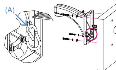
2. Pull the safety wire and cables through the Cap and rotate the Cap. Align one of Cap's screw holes (B) with the hole of mount (C). Fasten hexagonal screw (C) with proper tool.
