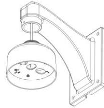
FIGURE 2-1: ASSEMBLE THE PENDANT MOUNT WITH WALL MOUNT
