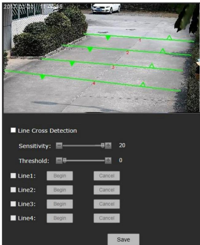
Figure 4-50 Line Cross Detection
