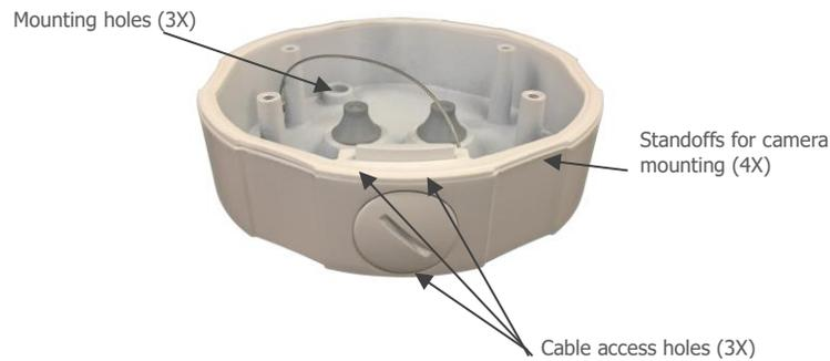
Loosen the three screws on the clear dome assembly to remove the clear bubble. Note that there is a bag of desiccant inserted in the camera assembly; do NOT remove this. Secure the camera dome to the standoffs in the back box using the screws and washers provided in the accessory kit.
