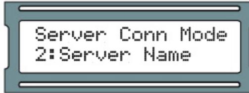
5. Using the white up and down buttons on the Panel, locate and set the indicating arrow on the LCD screen to 'Server name' and then press the ENTER button.
