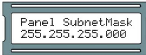
12. With the full subnetmask completed on the LCD screen, ensure you are in VIEW mode (indicated by positional value blinking between value and blank) and then press the ESC button.
