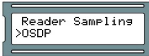
4. You will now choose an OSDP address to make changes or test. If you're not sure what the address is you should start with 00. Using the white up and down buttons on the Panel, locate the address you want to change or test and press the Enter button.
