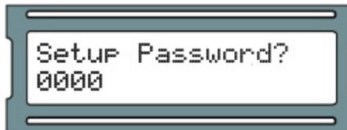
2. If the panel is using the default password ('0000'), press the ESC button. You should then be presented with a message on the LCD screen stating 'ACCESS GRANTED'. If the panel already has a password, you will enter it now using the white up and down buttons and the ENTER button (Note: If there is no configuration activity for 60 seconds, the Panel will perform a forced logout).
