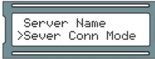
4. Now on the 'SERVER CONN MODE' screen, press the white up or down buttons until the arrow on the LCD screen is indicating '1: Server IP' is selected and press the ESC button.
