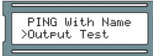
4. Press the white up or down buttons to move the cursor over the Output you'd like to test. Press ENTER and the highlighted zero will change to a 1, and the Output will be triggered. Press ENTER again to disengage the Output. When you are done testing, press the ESC button.
