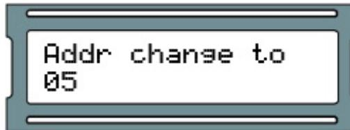
10. If successful, you will see the old and new address displayed with the message Success. Record the new address and press the ESC button to leave this menu. Timeout will be displayed if the address you were trying to change from was unreachable.
