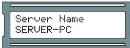
7. With full server name completed on the LCD screen, ensure you are in VIEW mode (indicated by positional value blinking between value and blank) and then press the ESC button.
