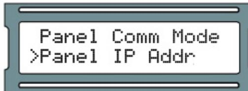
7. Using the white buttons for left and right movement as well as using them for changing numerical values for each position of the IP address of the Panel and using the ENTER button to switch between EDIT mode (position blinking between value and solid black) and VIEW mode (position blinking between value and blank), enter the full Panel IP address.
