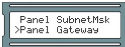
15. Using the white buttons for left and right movement as well as using them for changing numerical values for each position of the Panel gateway and using the ENTER button to switch between EDIT mode (position blinking between value and solid black) and VIEW mode (position blinking between value and blank), enter the full Panel gateway.
