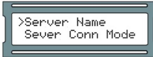
6. Using the white buttons for left and right movement as well as using them for changing alphabetical, numerical, and symbol values for each position of the server name and using the ENTER button to switch between EDIT mode (position blinking between value and solid black) and VIEW mode (position blinking between value and blank), enter the full server name (up to 16 characters).
