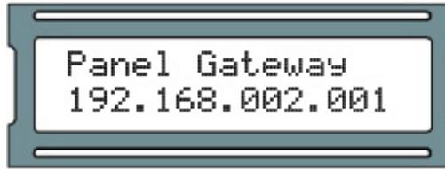
16. With full Panel gateway completed on the LCD screen, ensure you are in VIEW mode (indicated by positional value blinking between value and blank) and then press the ESC button.
