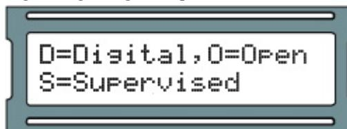
5. If you have any Input devices such as door contacts or REX devices, the Panel will beep and show you which Inputs are active. Inactive Inputs are 'DO' and active Inputs are 'DC'. If you're testing a door contact, open and close the door and monitor the Input change. When you are done testing, press the ESC button.
