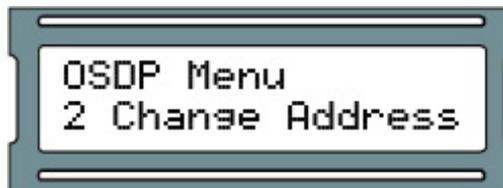
9. You can now choose the new address. Use the white up and down buttons on the Panel to increment/decrement the address. When you are ready to choose the address, press the ENTER button.
