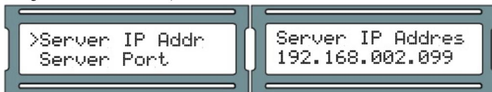
8. With full the IP address completed on the LCD screen, ensure you are in VIEW mode (indicated by positional value blinking between value and blank) and then press the ESC button.
