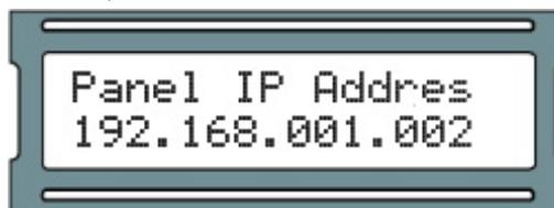
8. With full IP address completed on the LCD screen, ensure you are in VIEW mode (indicated by positional value blinking between value and blank) and then press the ESC button.
