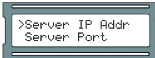
7. Using the white buttons for left and right movement as well as using them for changing numerical values for each position of the IP address of the server and using the ENTER button to switch between EDIT mode (position blinking between value and solid black) and VIEW mode (position blinking between value and blank), enter the full server IP address.
