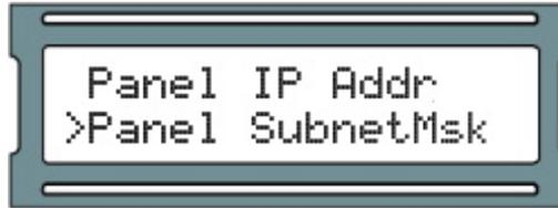
11. Using the white buttons for left and right movement as well as using them for changing numerical values for each position of the Subnetmask of the Panel and using the ENTER button to switch between EDIT mode (position blinking between value and solid black) and VIEW mode (position blinking between value and blank), enter the full Panel subnetmask.
