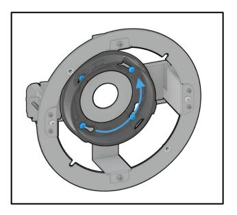
4. Insert the In-Ceiling Bracket/Base assembly into the hole in the ceiling.
