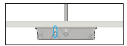
2. Align the two lock screws on the Solo Fixture with the double dot indicators on the installed Network Hub.
