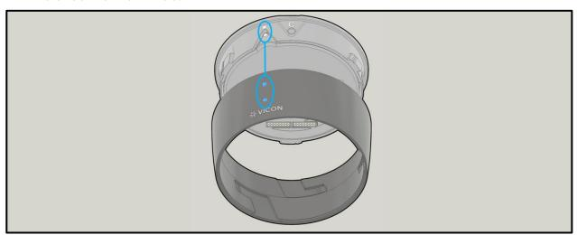
3. Twist the Solo Fixture to the right to lock it into place. The Vicon logo on the Solo Fixture is now aligned with the Base's centerline ("C").
