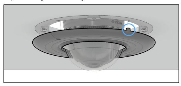
NOTE: The fingers on the inner diameter lock into the grooves on the Camera Sensor.
