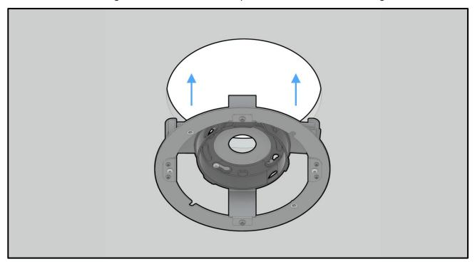
5. Use the T20 Torx Wrench to tighten the locking screws; as the screws tighten, the locking wings unfold and lower until they hit the ceiling to secure the bracket to the ceiling.
